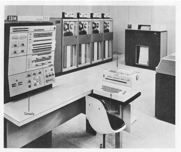
IBM System/360 Model 40 Console, Console Printer, and Keyboard
